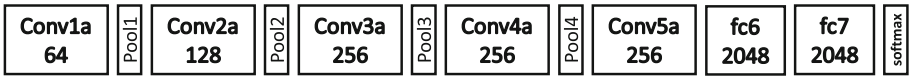
Fig. 4. 3D CNN architecture. The network has 5 convolutional, 5 max-pooling, and 2 fully connected layers, followed by a softmax output layer. The number of filter in each layer is denoted at the bottom of each box. Each fully connected layer has 2048 output units.
